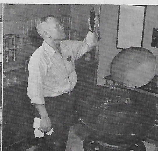
(L-R) Adolphe St. Marie gauges a tank of Poso crude prior to shipment. Stephen Keithley manipulates the controlling steam throttle of a main line pump to start the crude flowing. Lawrence Marston removes sample of crude from centrifuge to determine its water cut and sediment content.
