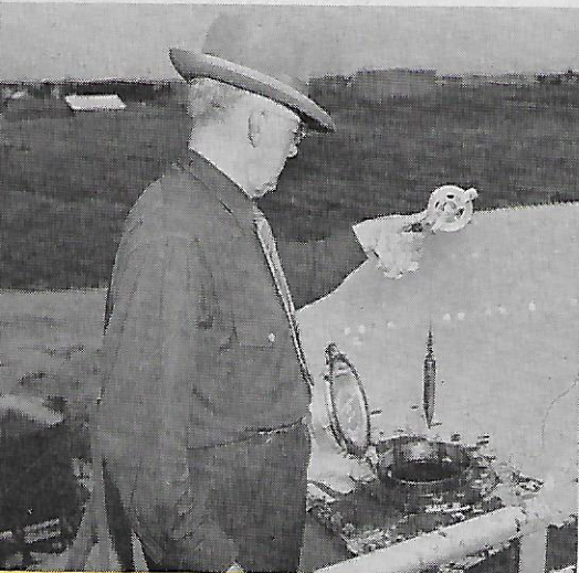
(L-R) Adolphe St. Marie gauges a tank of Poso crude prior to shipment. Stephen Keithley manipulates the controlling steam throttle of a main line pump to start the crude flowing. Lawrence Marston removes sample of crude from centrifuge to determine its water cut and sediment content.
